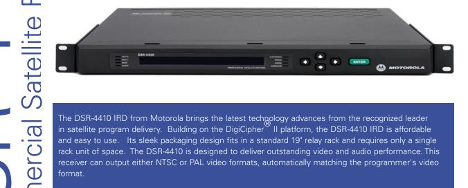
With a variable front-end and bypass capabilities, the DSR-4410 is ideally suited for network conversion from analog to digital. Full VBI reinsertion on lines 10 - 22 for SID/AMOL I & II and NABTS is standard on the DSR-4410. Equipped with DVB-ASI input and output, the DSR-4410 is ready to connect to the rest of your head-end equipment.
