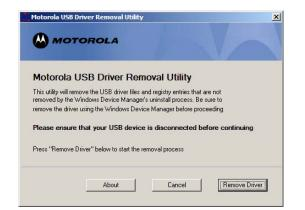
The SURFboard Cable Modem USB Driver Removal window is displayed. *Be sure the USB cable is disconnected.*
