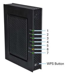
The SBG941 front panel LED indicators provide the following status information for power, communications, and errors:
