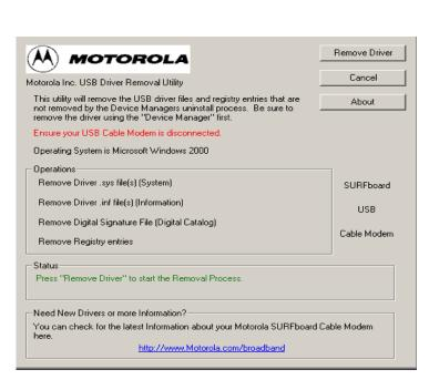
The USB cable must be disconnected before running the REMOVE utility.
