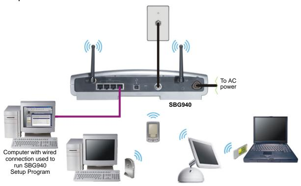
To set up the SBG940, on a computer wired to the SBG940 over Ethernet or USB, perform the procedures in "Setting Up Your Wireless LAN". Do not attempt to configure the SBG940 over a wireless connection.
