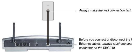
Before you connect or disconnect the USB or Ethernet cables, always touch the coaxial cable connector on the SBG940.
